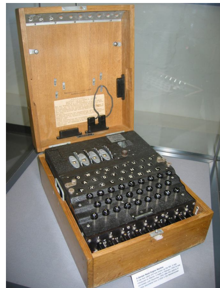
German Naval Enigma machine
